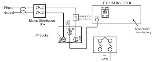
\*(1. Point to point wiring required. 2. Max. 0.8 PF of rated capacity bulb load)
